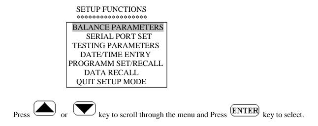
**BALANCE PARAMETERS** : Use this menu to change parameters required for the functioning of the balance.
