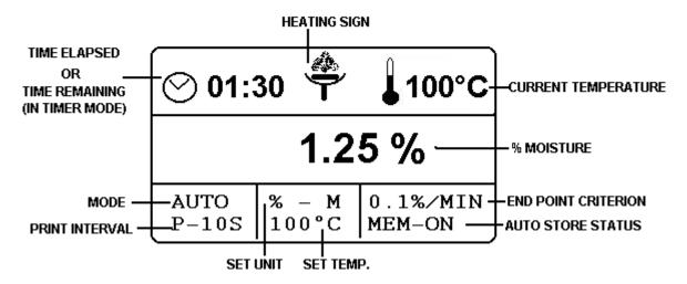
Balance will continuously display % moisture (or whichever unit is selected) along with current temperature and elapsed time ( or remaining time in TIMER mode) along with other set parameters.
