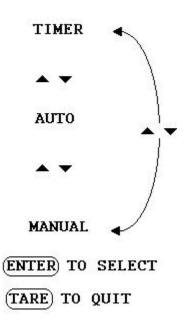
Use ▲ or ▼ keys to change from 3 min. 120 min and press ENTER key to save. This is applicable only in TIMER MODE.
