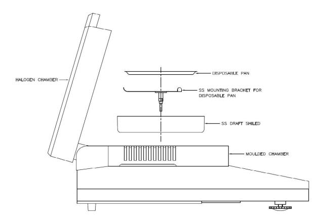
Place the instrument on a sturdy levelled surface. Level indicator is placed on the rear side of the balance. Turn the front knob screws to level the balance, if required.
