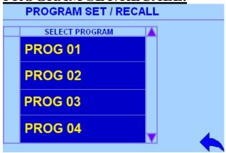
Moisture balance has a provision for storing 10 drying methods (**PRG-1 to PRG-10**) in memory for easy recall. All the Testing Parameters i.e., Measurement unit, Measurement Mode, Temperature, Test Time, End point, Auto Store and Print interval can be modified and stored in individual memory for later use.
