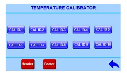
10 calibration IDs, header and footer details can be set.
