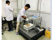
Highly advanced Mass Comparators for the testing of 1mg ~ 20kg weights up to E1 class
