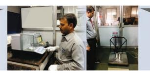
Contech metrology engineer calibrating industrial weighing scale using appropriate standard weights
